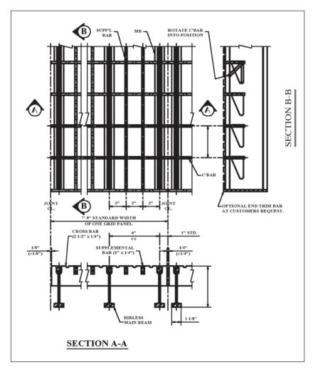
WARNING: Uncoated-weathering steel provides the best skid resistant open grid surface. Galvanized or painted coatings can reduce the skid resistance. Vertical and/or horizontal curves on the bridge decking can increase lateral forces on vehicles, further reducing skid resistance efficiency. It is recommended that lane changes be prohibited and appropriate speed limits be strictly enforced to promote safety. Various studies are available upon request.
