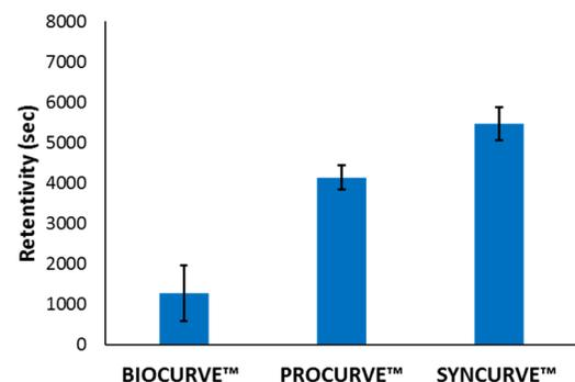
**Figure 1.** Twin disc testing results for SYNCURVE™, PROCURVE™ and BIOCURVE™.
