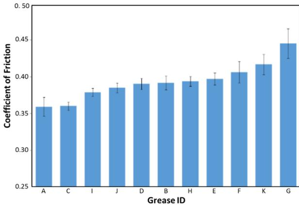
**Figure 2.** Average friction level for different greases 3.2-4.8 km from application site. Greases E and F were labelled biodegradable by the suppliers. Grease A is PROCURVE™.<sup>ii</sup>
