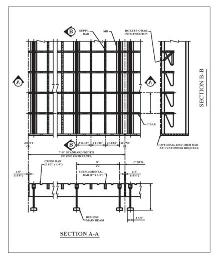
WARNING: Uncoated-weathering steel provides the best skid resistant open grid surface. Galvanized or painted coatings can reduce the skid resistance. Vertical and/or horizontal curves on the bridge decking can increase lateral forces on vehicles, further reducing skid resistance efficiency. It is recommended that lane changes be prohibited and appropriate speed limits be strictly enforced to promote safety. Various studies are available upon request.
